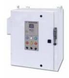
The E7/Bypass package is a 3-contactor style bypass, allowing motor operation from either the drive or across the line. This facilitates drive maintenance while the motor continues to operate. The E7 and E7/Bypass have been designed for flexibility in providing the features and options commonly specified by facility designers.
